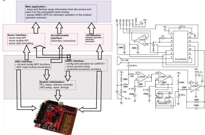
The main application running on the embedded linux machine on the robot includes an adapting layer to support the interface with the sonar interface module and the support for data acquisition used in the sensor fusion stage for the SLAM algorithm. The main architecture of the real time control application was enhanced to include the new functionality. The next image synthesizes the final application layers.
